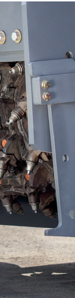
3 | - 4 | When fully lowered, the hydraulically adjustable edge protector reliably closes the drum housing while enabling the cold milling machine to be driven along obstacles when raised.
