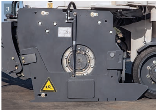
3 | - 4 | When fully lowered, the hydraulically adjustable edge protector reliably closes the drum housing while enabling the cold milling machine to be driven along obstacles when raised.
